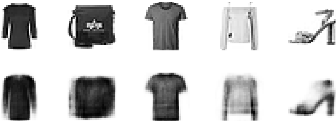
Figure 17-4. Original images (top) and their reconstructions (bottom)
